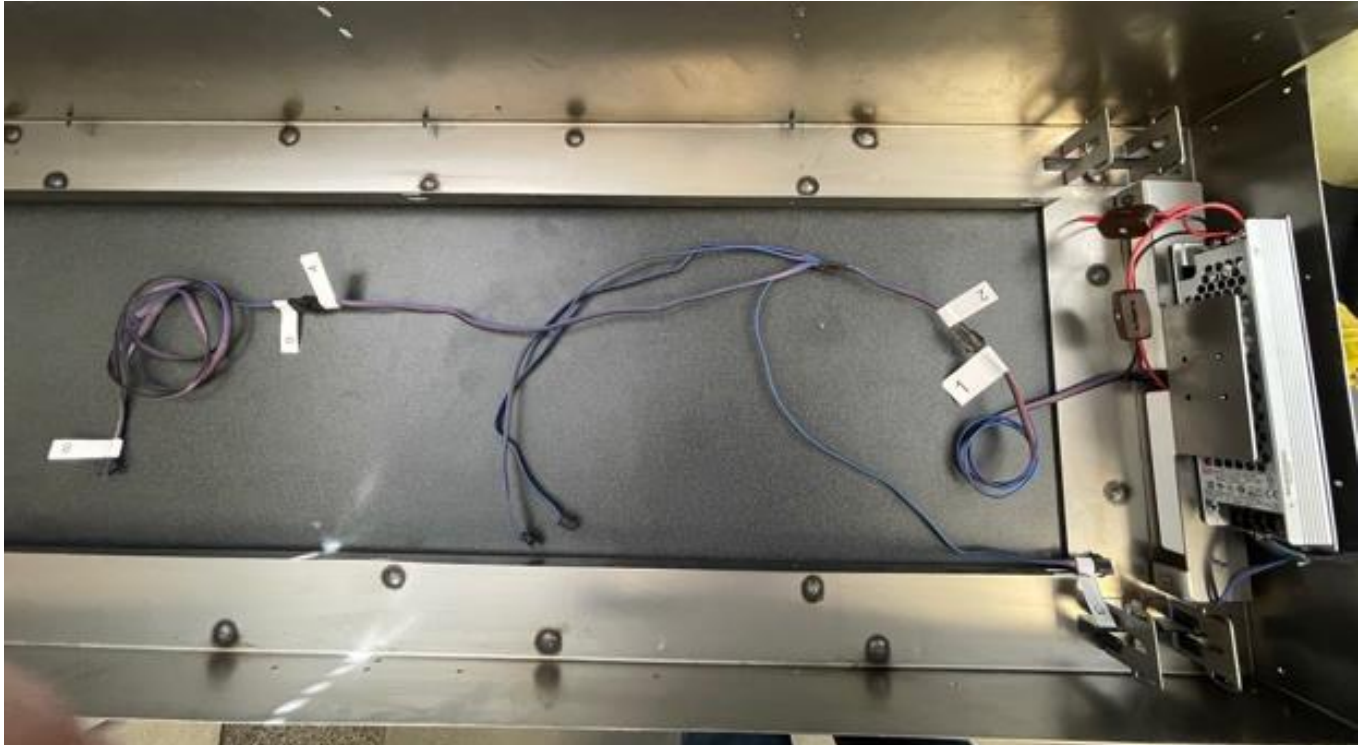
Connecting LED controller terminal to 1 to 4 splitter
