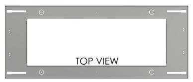
If you are not installing the Rock Tray or LED Light Tray you will have to mark the locations of the holes and drill them. The recommended locations are shown in the chart on the next page for each specific model.
